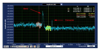
Use convenient cursor tools to measure and examine scatter level and reflection events to measure RL and IL for closely spaced events.
