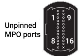
Figure 11: MPO-24 port configuration with 16 fibers
