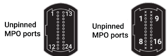
Figure 18: MPO-24 connectors with 24 fibers (left) or 16 fibers (right)
